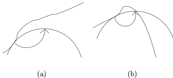
Figure 4.1: Use of (a) strong-sense and (b) weak-sense auxiliary functions for function optimisation
